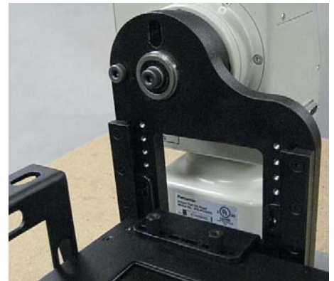
Close-up of the Dynamic Balancing Cradle shows two-axis adjustability for setting exact dynamic balance throughout the tilt range
